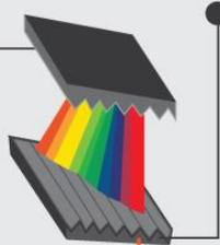
**2 The pulse is stretched, which reduces its peak power**
