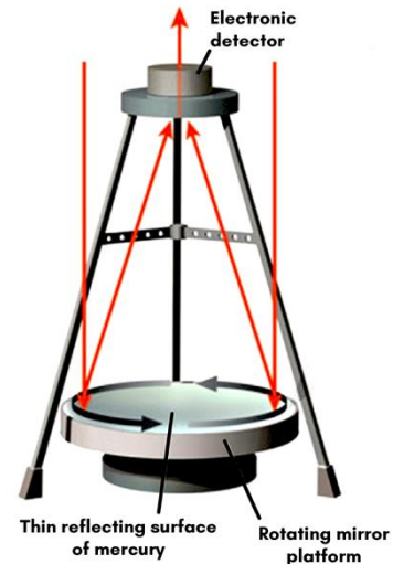
How liquid-mirror telescopes work
